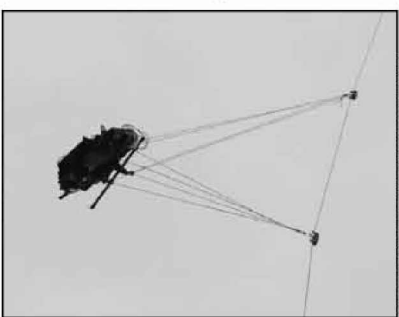
This camera is attached to a kite line. The flier can lift the camera high above the ground and use a remote control to make photographs of the subject.
